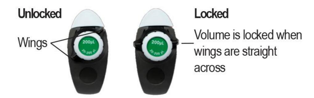
2. With the mechanism unlocked, orient the pipette so you are looking at the digital volume indicator, then rotate the plunger button to change volume – counter-clockwise to increase, clockwise to decrease volume. The volume indicator is read from the top down and is color-coded in relation to where the decimal point should go.
